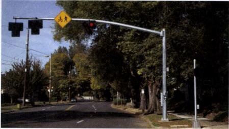
Pedestrian crossing facilities may range from flashing signage and striping (shown in the first image above) to pedestrian hybrid beacons (shown in the image above). A hybrid beacon would be considered for the five-lane highway section.
