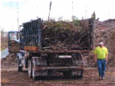
This 20-CY roll-off container has a tailgate (in open position). The load appears to be near top of truck sides and was estimated at 85 percent. The assessment was done from the ground; no monitor tower was used at this TDSR (see next photograph).
