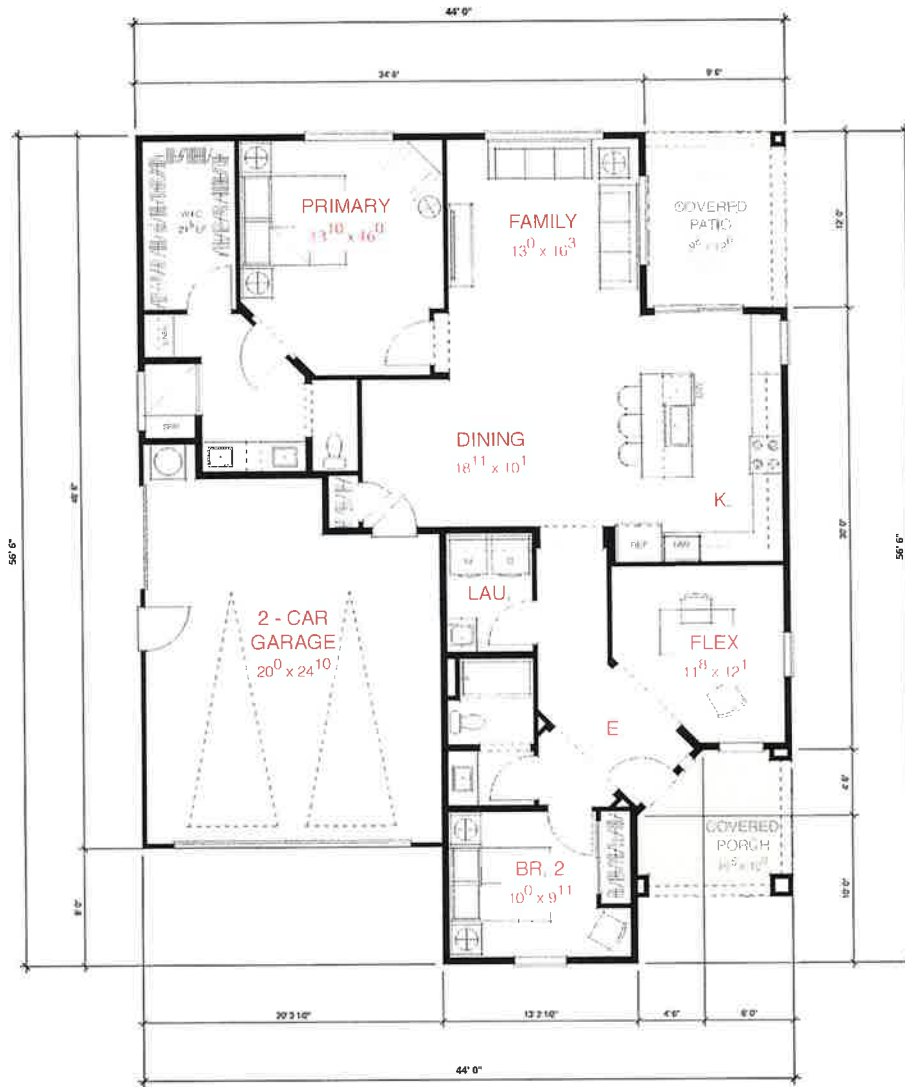
PLAN 3 | SCHEMATIC FLOOR PLAN | 1,579 SF
